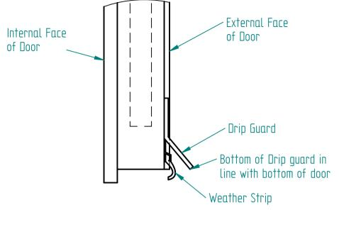
Locations are for illustration purpose only, weather kit should be positioned appropriatly for each individual door.
