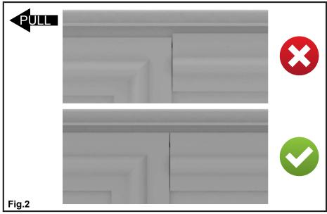
Make sure that the flanges at the top of the shutter doors are square to each other and that they run level to the frame (fig.2). If they are not square, pull the frame over until they are square. The frame can now be welded in place.
