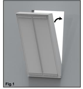
Insert one side of the glass unit into the shutter frame and then pivot the opposite side into place. Fix the glass unit to the shutter frame through the fixing holes provided.
